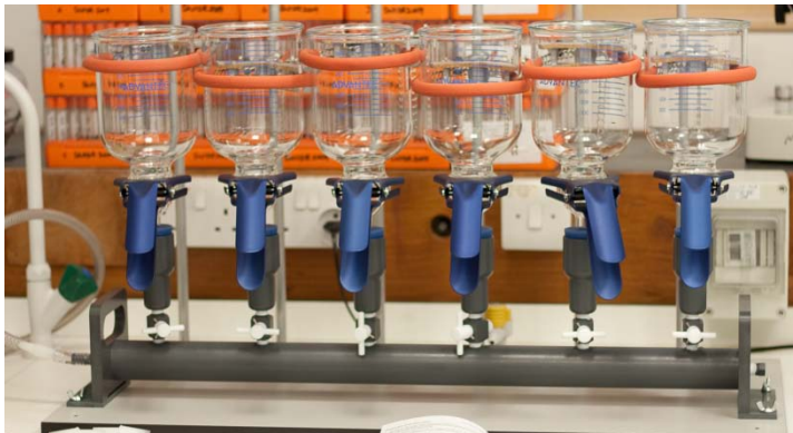
Figure 1 Water filtration system used on the JC80 cruise. One manifold with six glass containers with filters to sample the microorganisms in seawater was used. The glass containers were held in place with rubber bands (orange) and clamps (blue).
