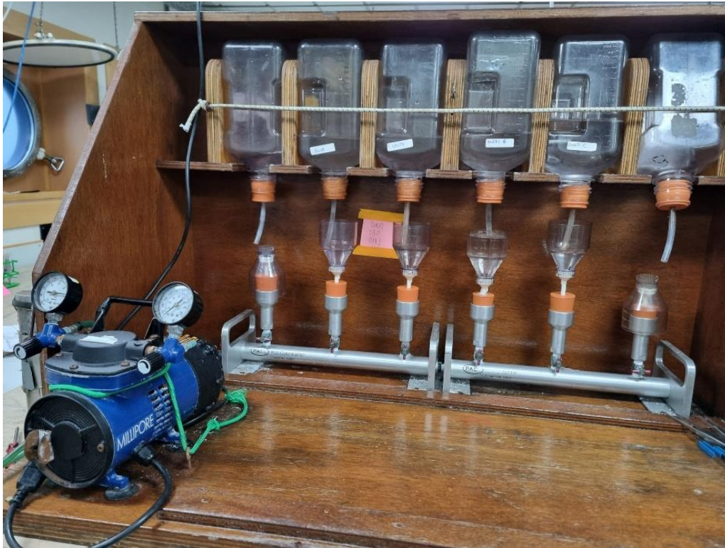
Figure 9.16: Filtration unit used on JC278
