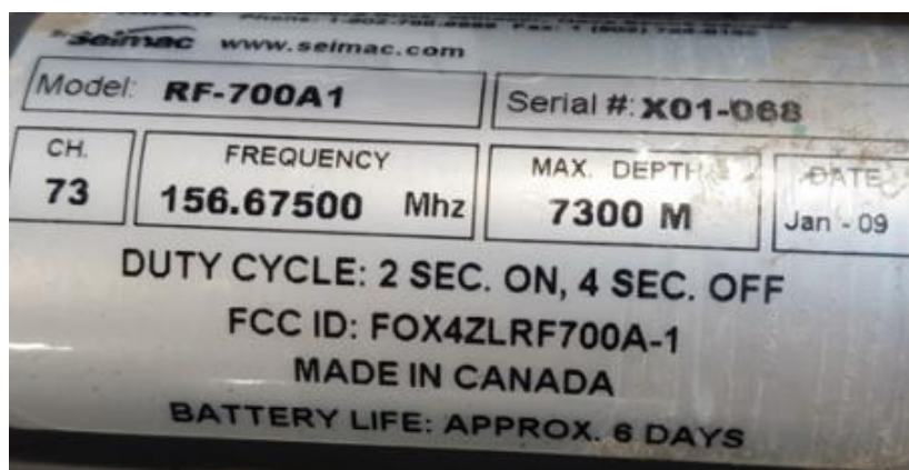
Figure 16.21: View of the VHF beacon information
