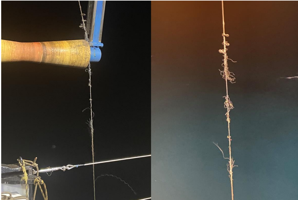
Figure 6.16: Damage to the deep tow cable after coming off the P-frame roller.
