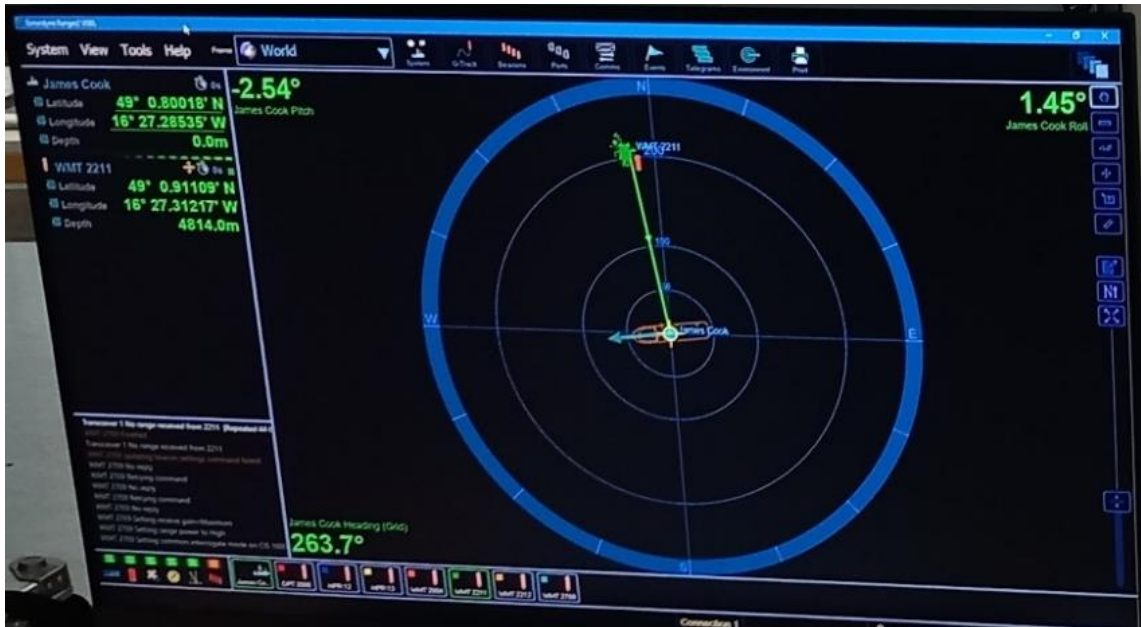
Figure 16.20: USBL positioning screen right before release
