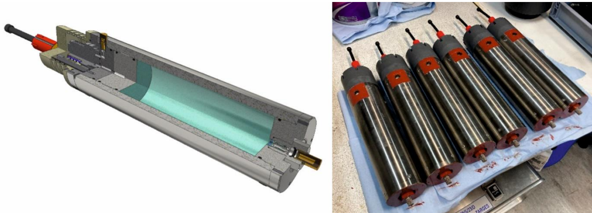
Figure 16.25: Section view of GTS v2.0 (left); 6x GTSs assembled and painted ready for deployment (right).
