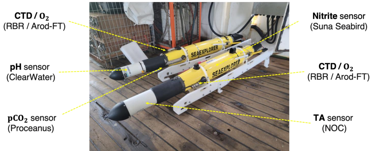
Figure 16.2: location of sensor payload on SEAEXPLORER gliders
