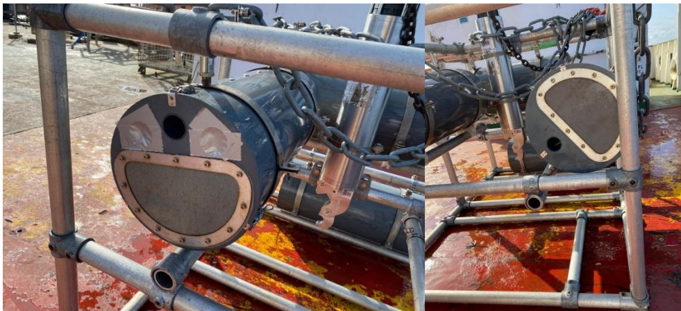
Figure 14.5: The amphipod trap as deployed in JC278-047. Left: Duct-tape added to two of the openings on the lid of TOP 2 to prevent sample loss on recovery. Right: inverted position of BOTTOM 2 on recovery.
