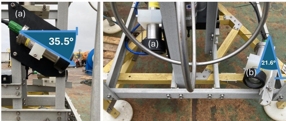
Figure 14.10: The mounting orientations of the camera (a) and flash (b).
