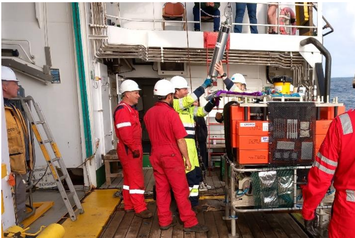
Figure 16.16: Connecting the acoustic release and synthetic rope (08:08)
