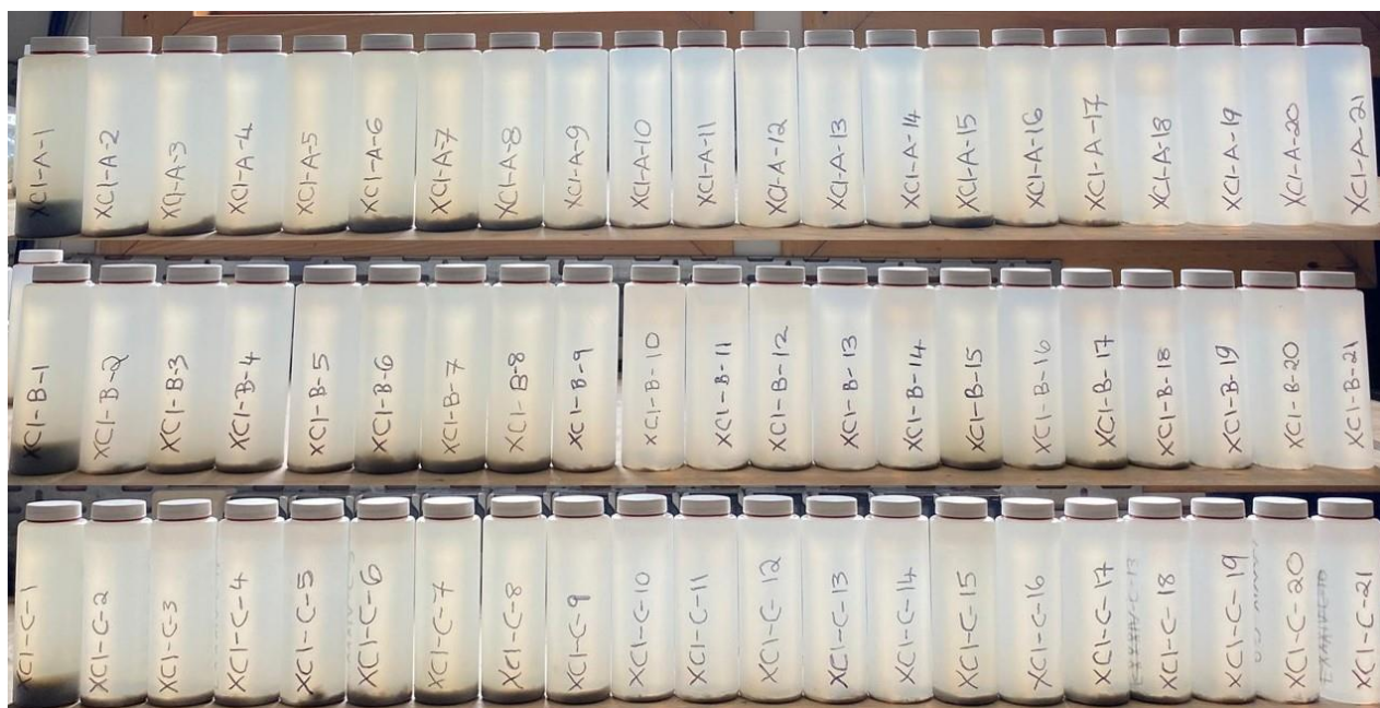
Figure 13.2: Photographs of sediment trap samples lined up in chronological order showing higher flux from the spring bloom towards the end of the deployment.
