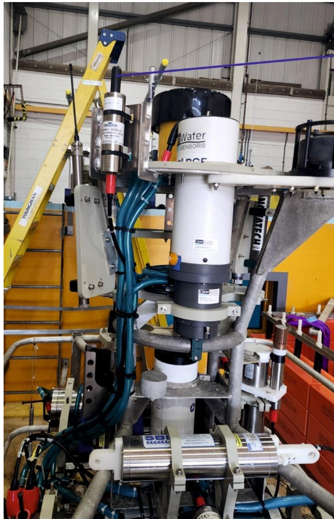
Figure 17.8: icListen HF hydrophone on EGIM lander.
