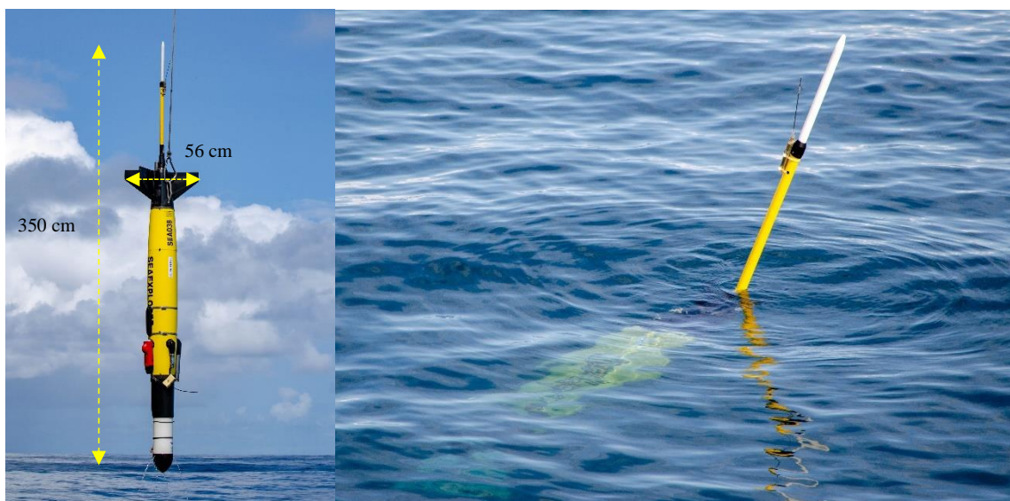
Figure 16.1: Photographs of a SEAEXPLORER on recovery and at the surface.
