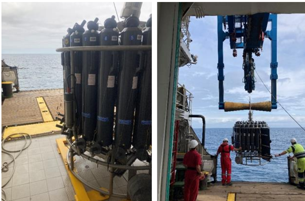
Figure 16.34: GTS 7 & 8 being deployed on the CTD frame
