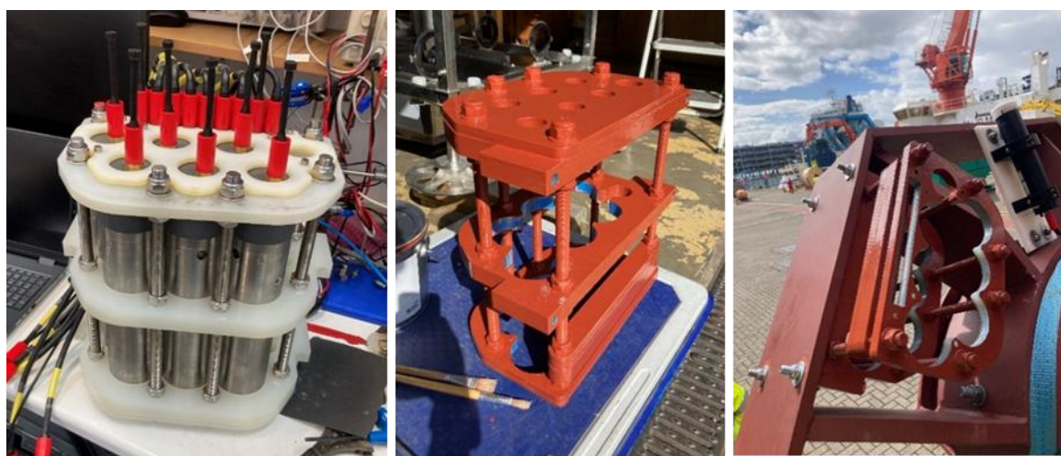
Figure 16.27: (left to right) GTS frame pre-paint; Frame painted with antifoul paint; Frame bolted to the keel of the buoy
