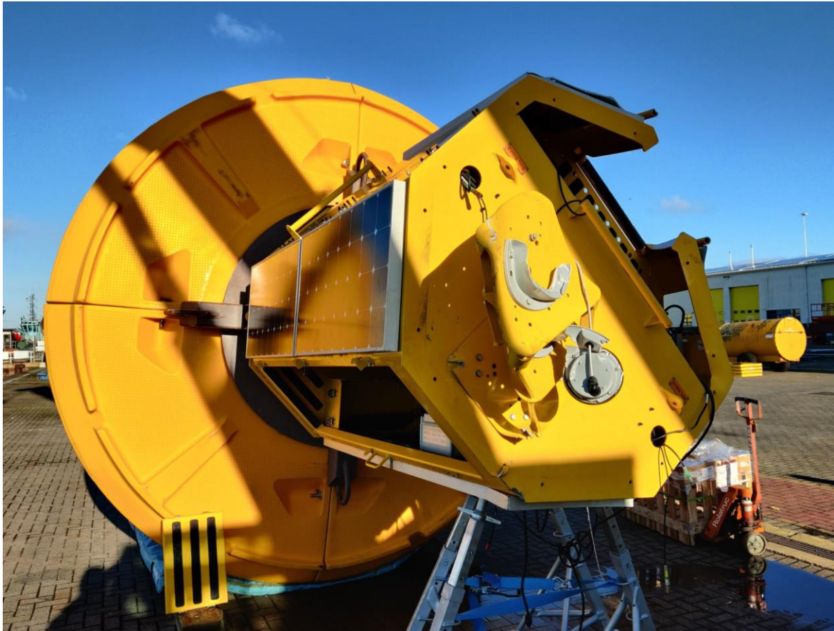
Figure 7.4: All sensors were lost from the mast of the buoy.
