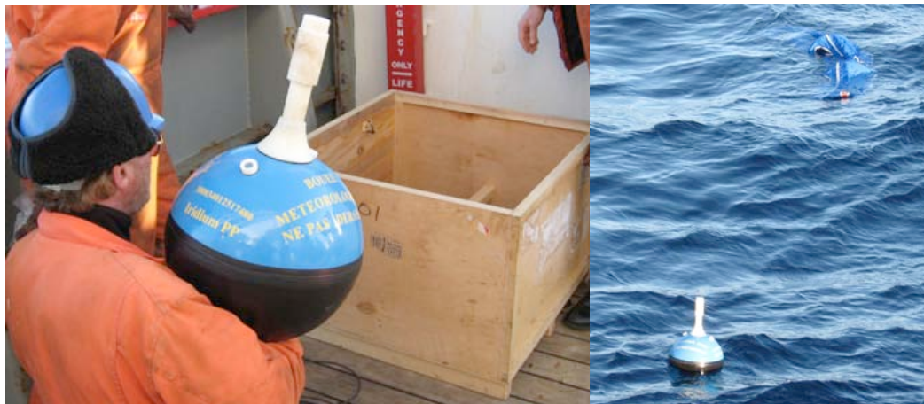
Figure 30 a) SAMS buoy taken out of crate; b) Buoy drifting away, with drogue unfurled.
