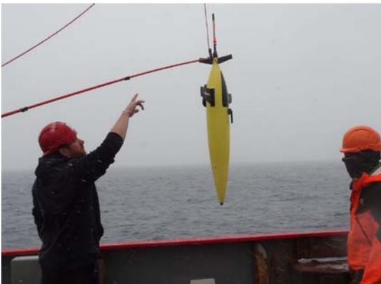
Figure 21: Glider deployment photo
