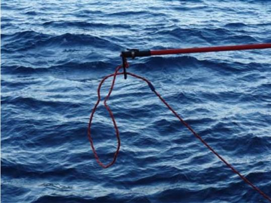
Figure 22: Glider recovery sling
