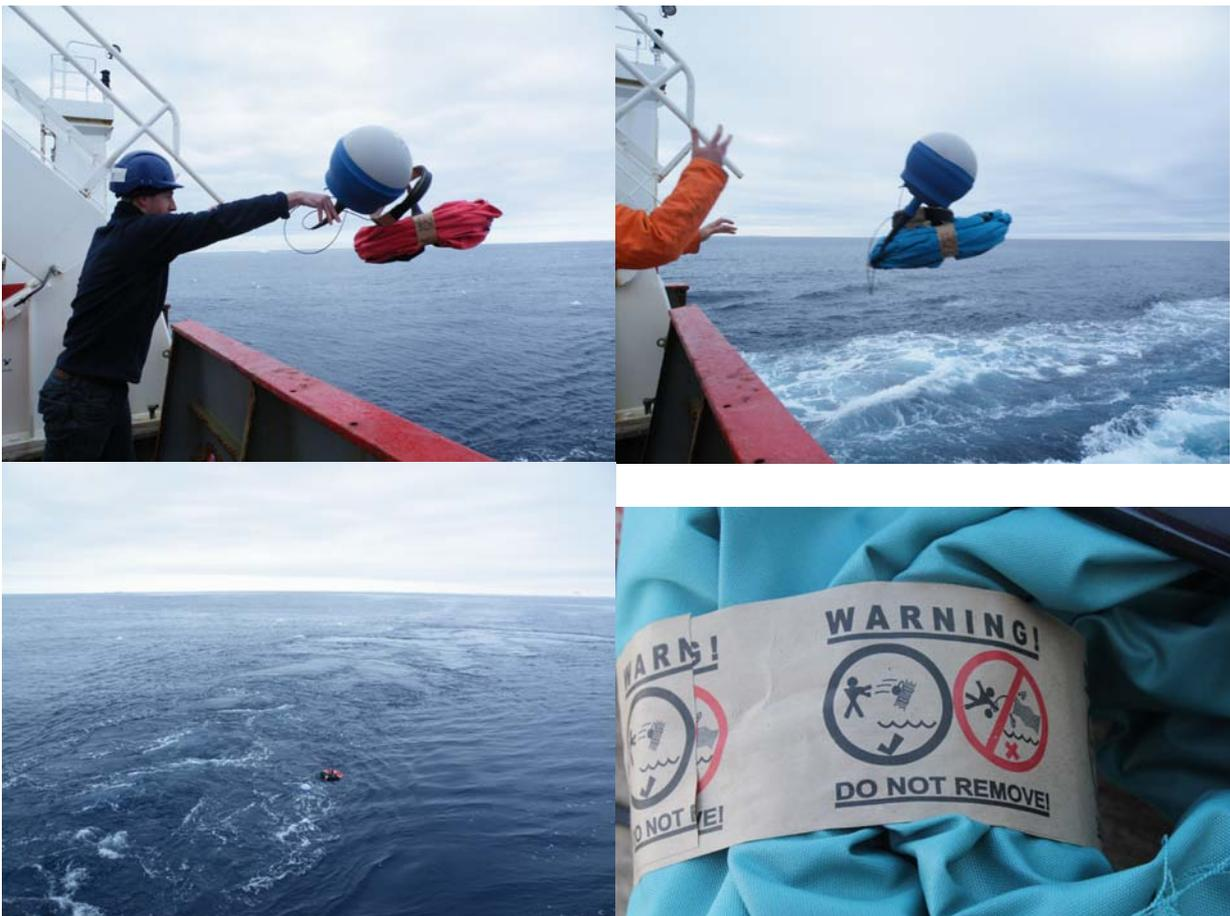
Figure 18: Drifter deployment from first section (start of WOCE SR04)
