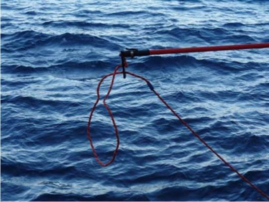
Figure 22: Glider recovery sling
