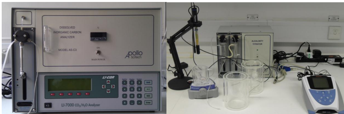
Figure 1: Apollo AS-C3 (left) and AS-ALK2 (right) used for the determination of Dissolved Inorganic Carbon and Total Alkalinity.
