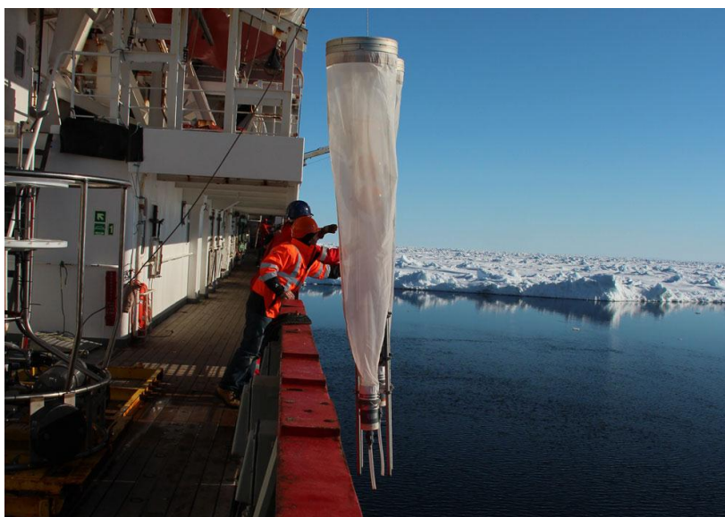
Plate 1: Deployment of the motion-compensated Bongo net
