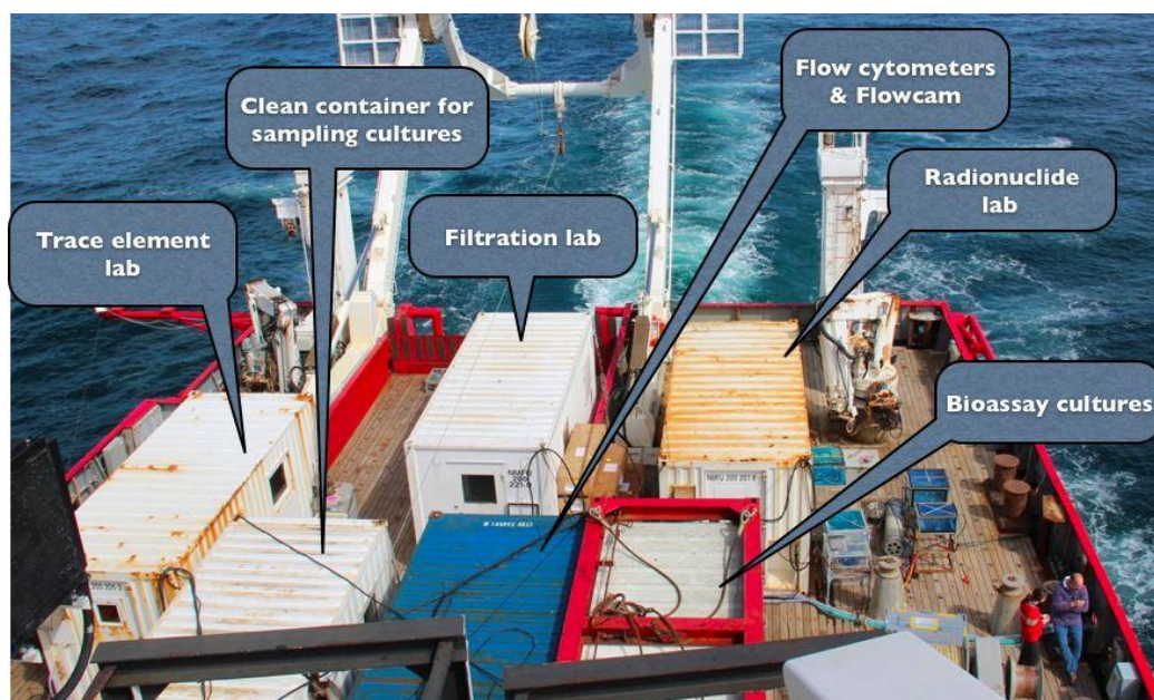
View of the aft deck of the JCR showing positions of the laboratory containers and deck incubation tanks
