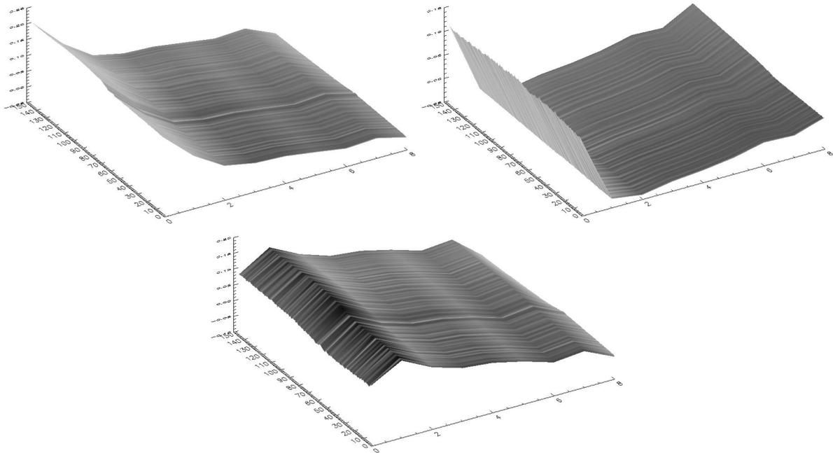
**Figure 3.** *ac/9 absorption spectra as determined by double casts. Top left is an absorption profile from an unfiltered ac/9, top right with 0.2µm filters ('CDOM cast') and bottom is the unfiltered minus the filtered profile ('particulate spectrum'). x = ac/9 channel number (wavelength), y = depth [m] and Z = absorption [m<sup>-1</sup>]*
