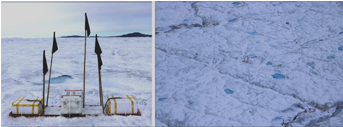
Fig. 10.1: Typical set-up of a pRES station. Left: final setup of the pRES station north. Right: view of the pRES station north from the helicopter.
