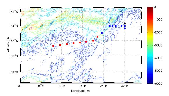
Figure 4.1: JC30 stations with LADCP profiles. The black square shows the position of the only station with a fully-working LADCP. The blues squares show stations with a weak beam and the red squares show the stations with a broken beam.
