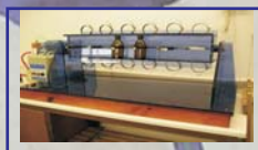
Fig 4: Predator exclusion experiments were carried out in triplicate bottles incubated with controls at in situ temperature for 24 hrs on a Plankton wheel
