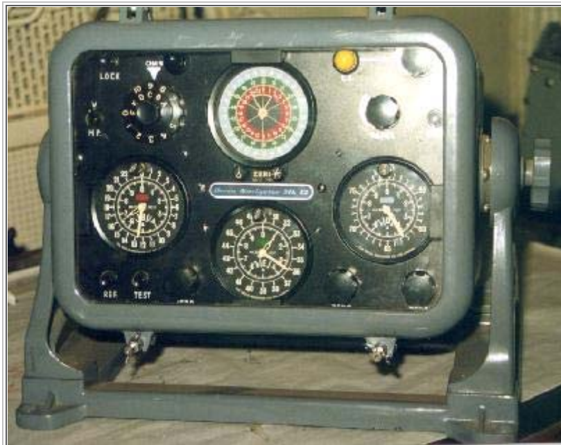
Here is an example of a Decca Mk12 decometer bowl which was donated to HMCS HAIDA Naval Historic Ship. One major change from the Mk V to the Mk XII system was the relocation of the chain selector switch from the receiver to the display unit. ( Photo by Jerry Proc )
