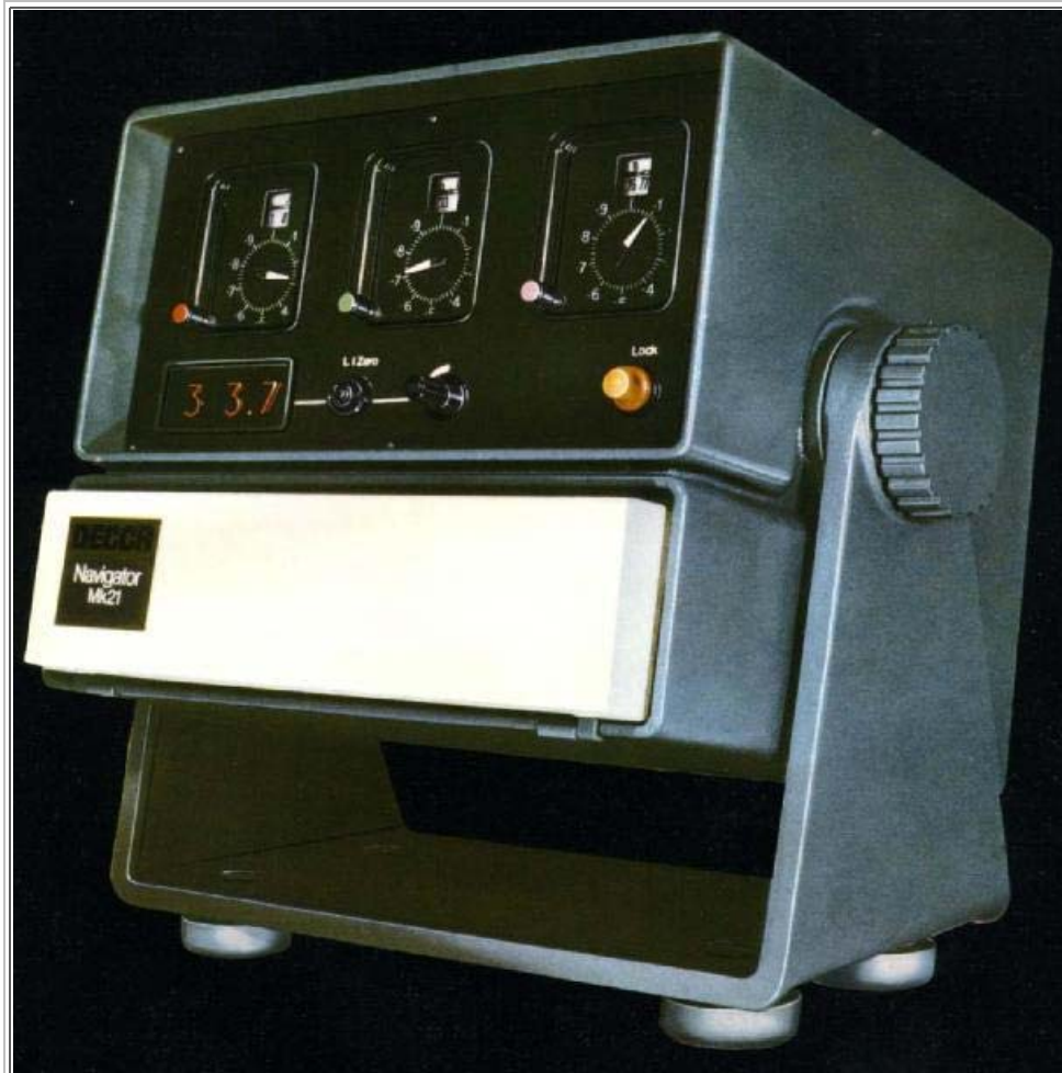
Introduced in November 1969, the Mark 21 was the first receiver where everything was contained in a single box unit. ( Photo from the collection of Walter Blanchard )
