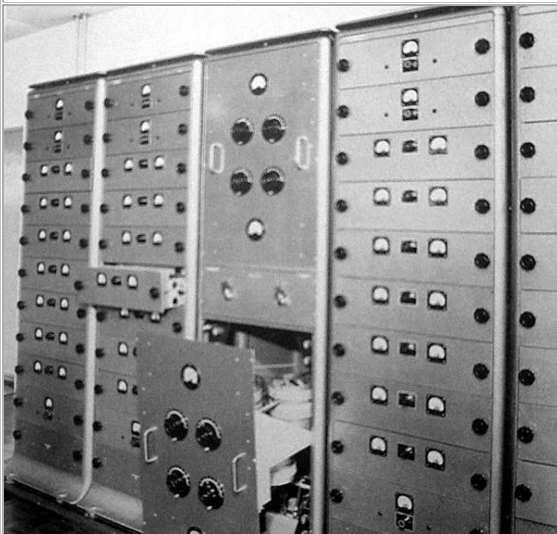
Each of the four transmitter racks in a station contains ( top to bottom) two drive units in parallel, six power amplifier units, one spare power amplifier and one spare drive unit. Only three out of four racks are shown. Two of these racks provide the normal pattern transmission and two provide Lane Identification (LI). At this Purple slave, two pairs of LI transmitters
