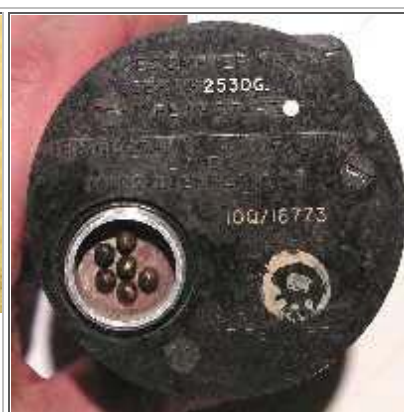
Rear view of GREEN Mk VIII aeronautical decometer. Type 274Z. P/N10Q16773 . (Photo courtesy Denis Chouinard)
