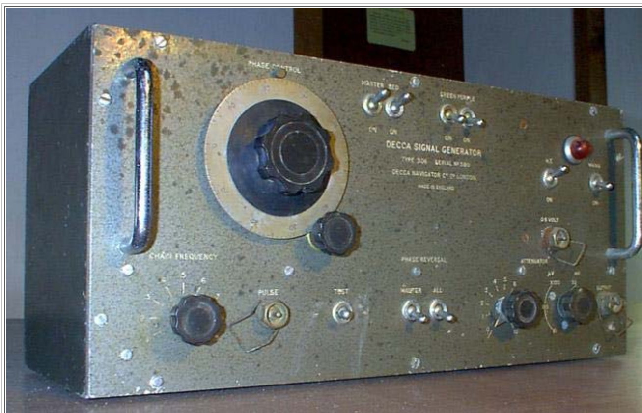
Decca Model 306 Signal Generator. These were used at the master stations to service the "Remote Monitor Receiver". The remote monitor was a modified MkV receiver, located about two to three miles from the station and connected to it by landline in such a way that the Decca signals could be displayed on the decometers in front of the watch keeper. A signal generator would also be held by the local marine service company who repaired shipboard Decca receivers. (Photo submitted by Santiago Insua <deccanavigator(at)mundo-r.com>)
