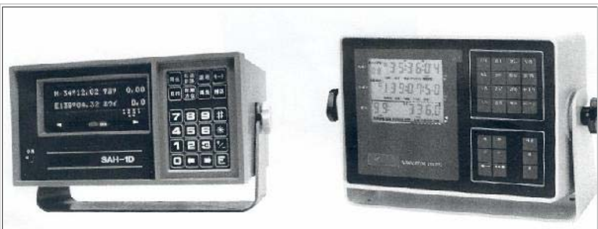
Two examples of direct reading Decca receivers are the Model SAH-1D (left) and the Navigator DR-702. The model SAH was sold to the Japanese market hence the reason for the Japanese characters on the keypad. ( Photo courtesy of the Sena Co, Ltd, Tokyo, Japan ).
