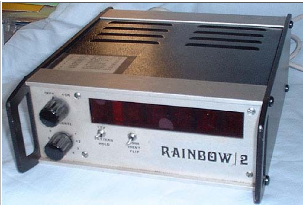
1975: A prototype of a microprocessor controlled Decca Navigator receiver designed by Sid Jones. ( Photo by Sid Jones )
