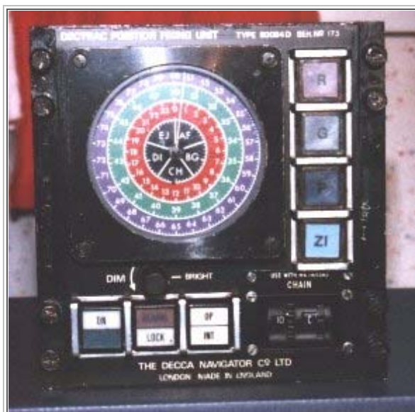
This was the airborne version of the Decca receiver called Dectrac Mk 19/15A3 s/n 175 built in 1980. (Courtesy of web page: http://perso.libertysurf.fr/webmeynier/aero/80084.htm )
