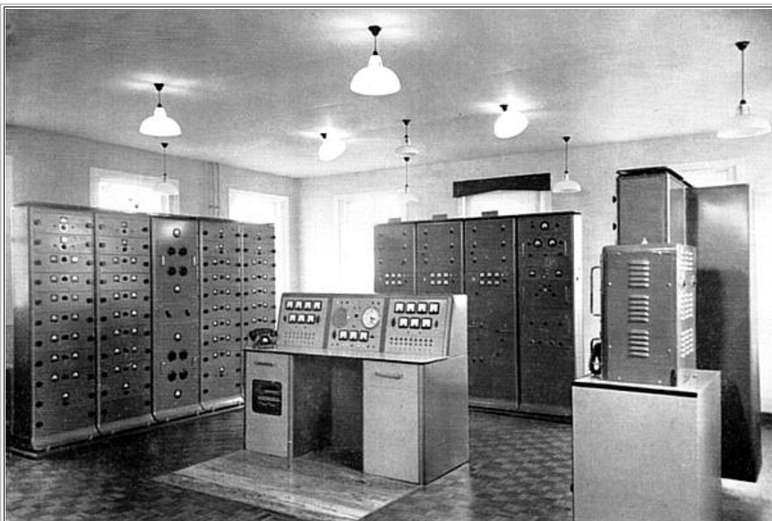
A typical Decca station using 820 series equipment. The monitoring desk is in the centre. (Photo courtesy Decca Navigator Company)
