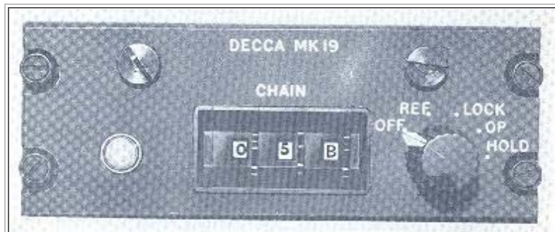
This is the receiver control unit ( Type 8954) for the Mk 19 airborne Decca receiver ( Photo courtesy Decca Navigator Company )
