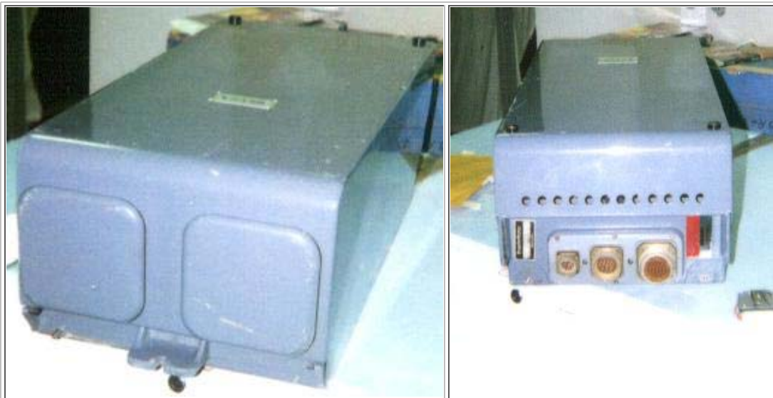
An example of a Decca Mk12 receiver. At the left is the top view; the bottom view is at the right. The chain monitoring receiver was a modified Mark12 unit. (Photos courtesy Maritime Museum of the Atlantic ).
