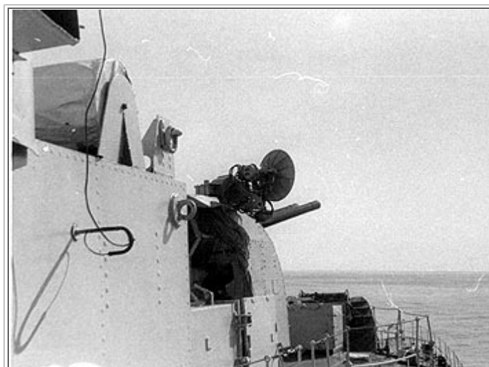
This detail shows the Decca Navigator antenna feedthrough assembly aboard HMCS Nootka in 1959. The assembly was made by Decca and was part of the rental kit. ( Photo courtesy of Gary Pollock )
