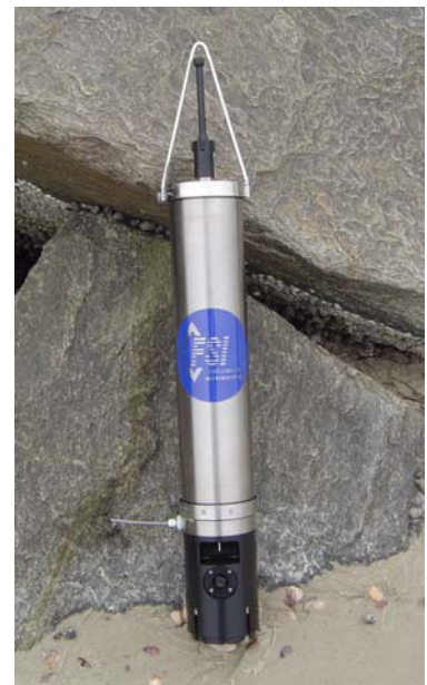
NXIC CTD Battery Power/Datalogging 7000 meter unit
