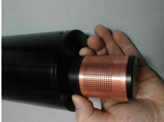
*Figure F-9: Mounting the guard*
