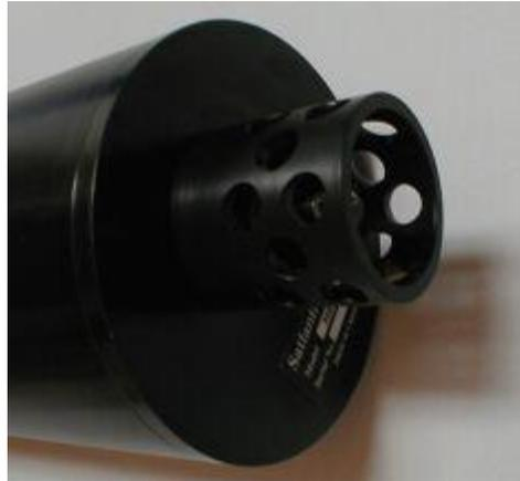
**Figure A-13: Standard Probe Guard Attached**
