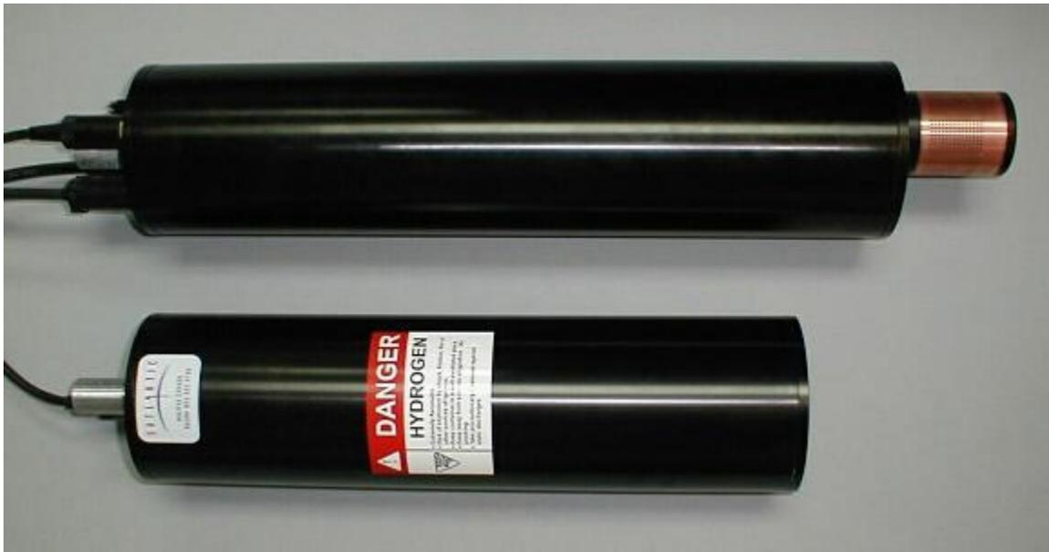
*Figure A-1: The MBARI-ISUS with Rechargeable Battery Pack*
