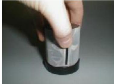
**Figure F-4: Insert a plastic shim**
