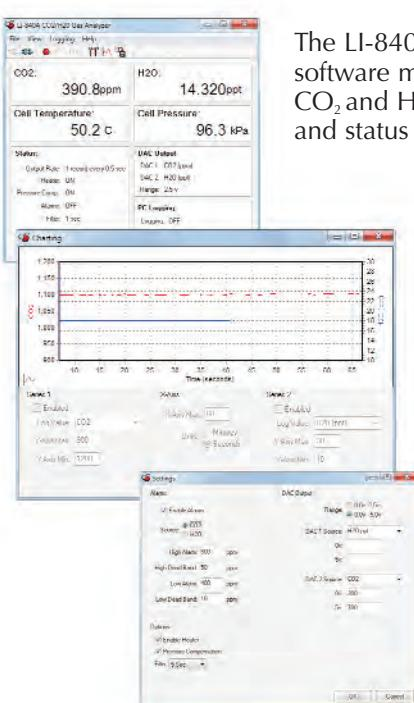
A choice of analog outputs (CO<sub>2</sub>, H<sub>2</sub>O, Temperature or Pressure) are selectable on either of the two user-scalable DAC channels. Linear analog voltage (0-2.5V, 0-5V) and current loop (4-20mA) outputs are available. A removable terminal strip allows easy connection of external recording devices such as the LI-COR LI-1400 Datalogger.
