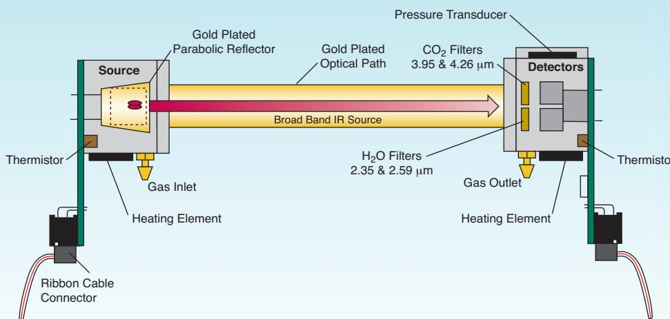
The LI-840A optical path is designed to achieve accurate CO<sub>2</sub> & H<sub>2</sub>O concentration measurements:
