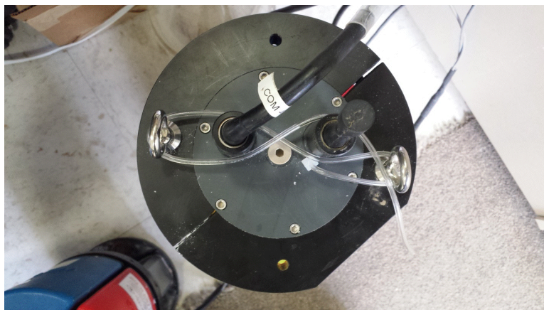
Figure 8 Eye bolts with exhaust tubing
