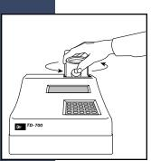
Seat the filter cylinder back in its chamber. With eight filters installed, the user can now switch between four different fluorescence analyses in seconds, just by rotating the cylinder.
