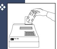
Lift the TD-700's sample chamber door and the unique filter cylinder slips out easily; it is ported to allow four different filter combinations.
