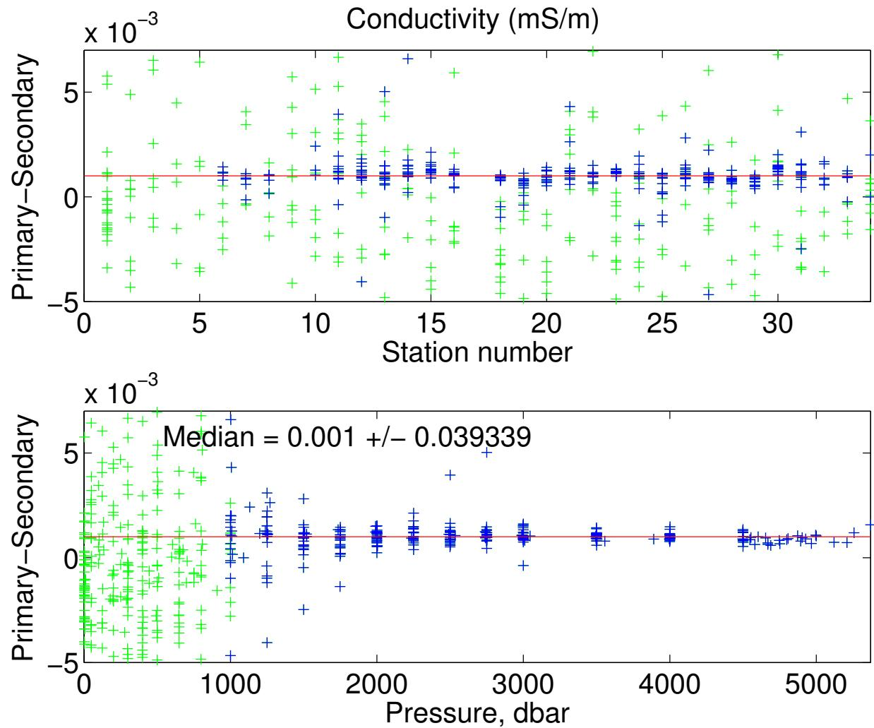
Figure 9: Conductivity (S/m) differences between sensors by station (top) and pressure (bottom). The red solid line represents the median with the red dashed representing the standard deviation.
