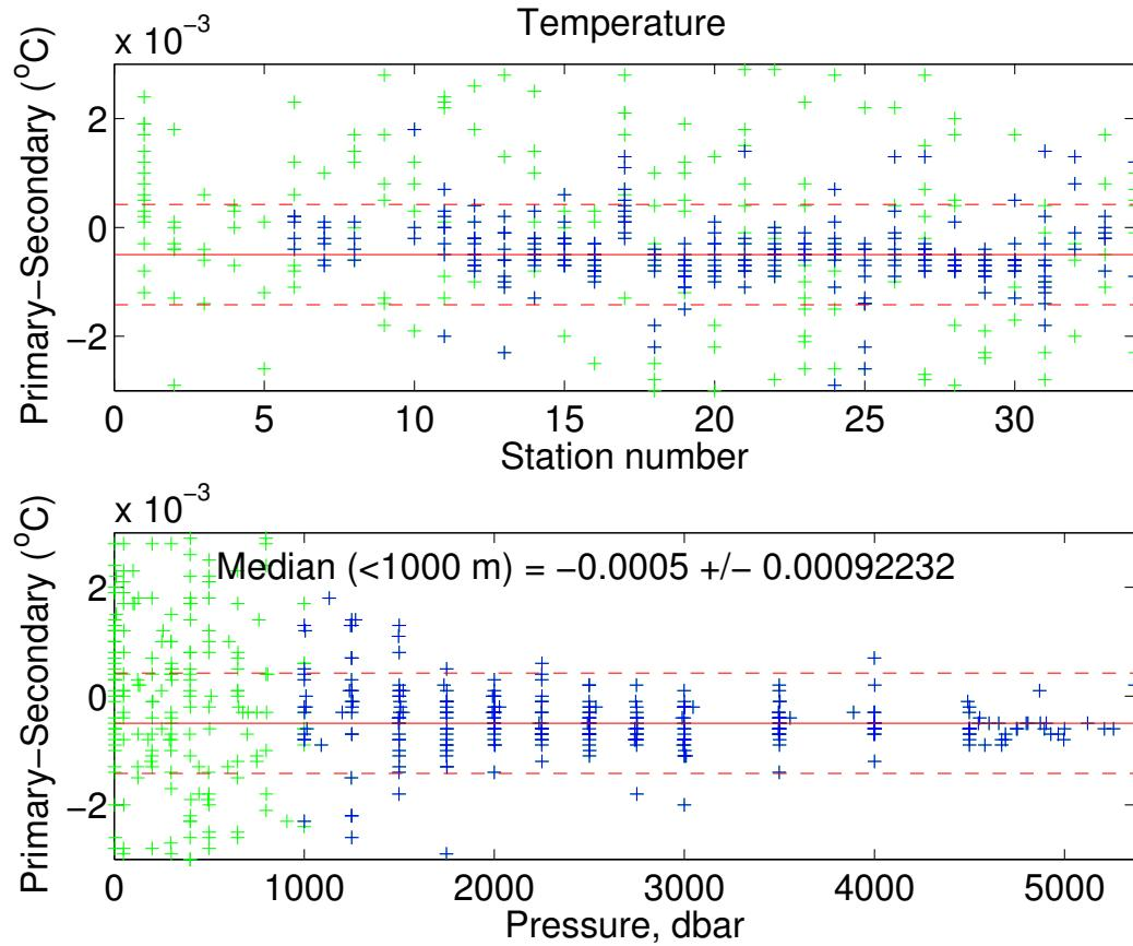
Figure 8: Temperature differences (after corrections) between sensors by station number (top) and pressure (bottom). The green represents the surface data down to 1000 dbar. The blue represents data below 1000 dbar. The red solid line represents the median with the red dashed representing the standard deviation (same for top and bottom).
