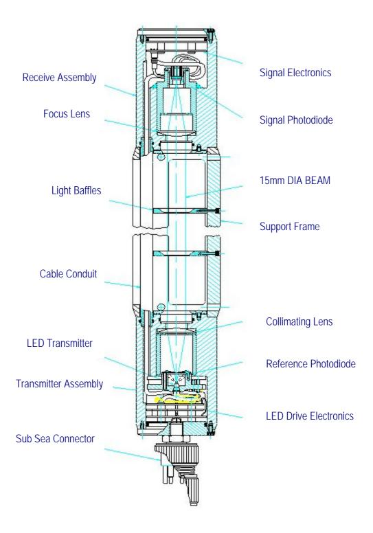
Figure 1 - ALPHAtracka II GA & Optical Layout
