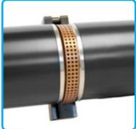
The SUNA V2 anti-fouling guard is a semi-circular piece of perforated copper attached to a plastic armature that fits into the sample chamber. It provides passive fouling prevention through the release of copper ions that inhibit biological growth in the area. The anti-fouling guard is a reliable and affordable approach to increase deployment time and decrease operating costs. It is intended for use in blue-ocean applications with low-to-no suspended sedimentation and/or low-to-no turbidity.
