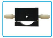
The SUNA V2 flow cell is designed to adapt the SUNA V2 for flow through operations on moorings with pumped flow, ship-board underway systems or for laboratory testing and calibration. The flow cell attaches to the SUNA V2 sample chamber and tightly seals against the optical chamber windows. Nylon barbed fittings are provided to connect the flow cell to available pumped flow.
