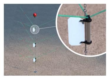
The most common Aquadopp application is classical in-line mooring use, where one or more instruments are mounted on a rope or cable that stretches from the bottom to a subsurface float.
