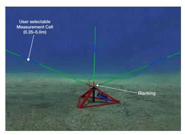
The Aquadopp® measures the Doppler shift occurring, when transmitting and receiving sound pulses transmitted along two or more narrow acoustic beams. This shift is proportional to the velocity component along those beams. By combining this information with the exact beam geometry, either 2D (2 beams) or 3D (3 beams) velocity is calculated.
