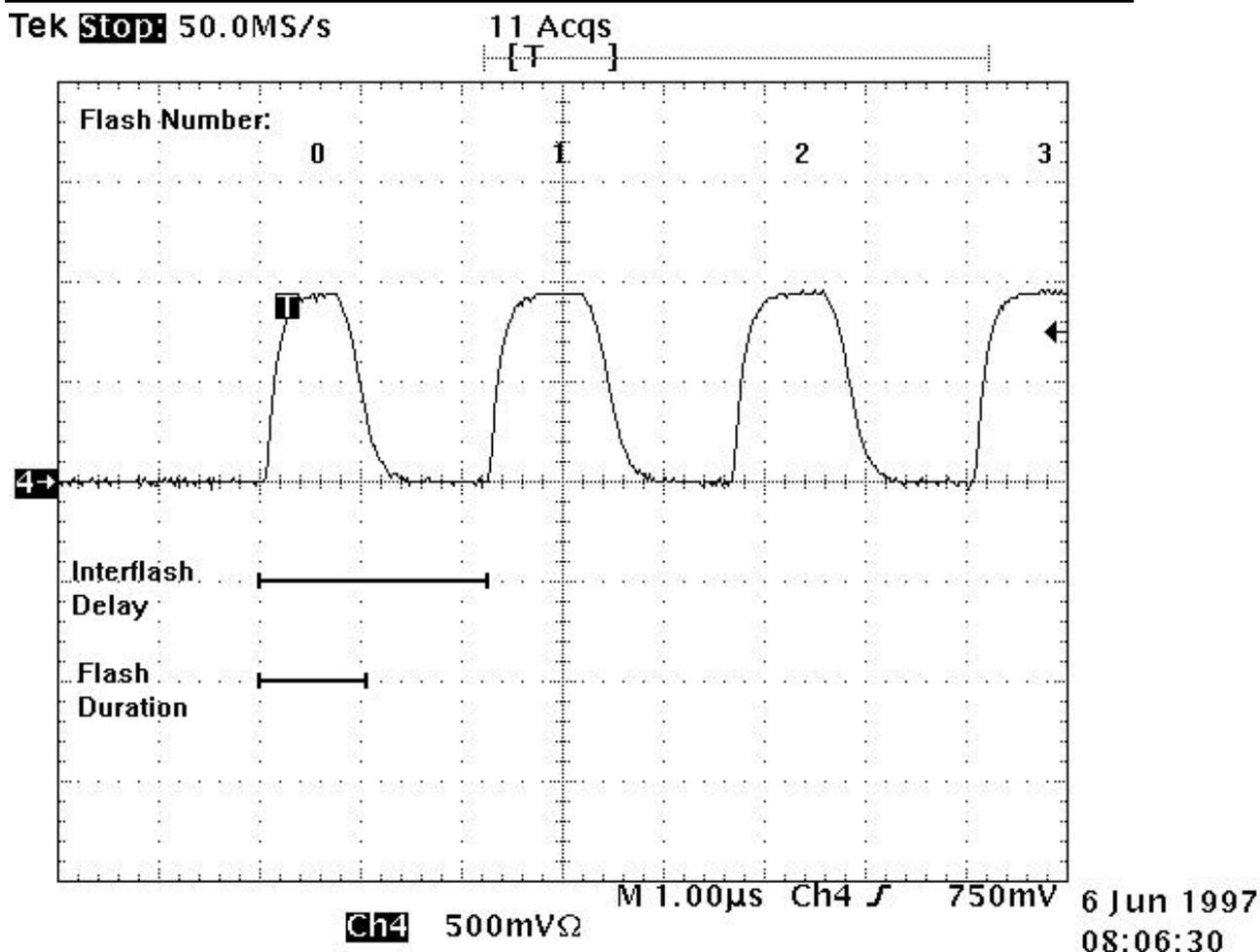
The flash duration (options 9 and D) is programmed in instrument units corresponding to clock cycles in the FPGA, as integers ranging from 4 to 100. The minimum value is set to 4 which gives a flash duration of 1.1µs, this being above 1 µs, which is the design specification for the detector electronics. Each additional integer increases in the flash duration value will increase the flash duration time by 60 ns.
