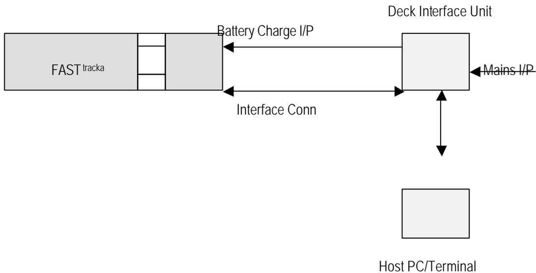
FAST<sup>tracka</sup> Interconnection Diagram for CTD operation and Pressure Sensor Option.
