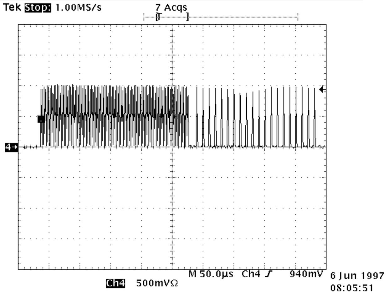
This above figure illustrates the actual timing of a flash sequence consisting of 100 saturation flashes and 20 relaxation flashes. The entire operation, as pictured, requires only 450  $\mu\text{s}$  for the programmed protocol. The Saturation group should be contained within a 250  $\mu\text{s}$  frame, and the relaxation group may be stretched into the order of milliseconds if desired. The above protocol was generated with the following parameters:
