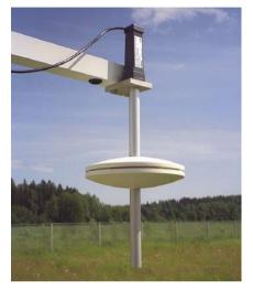
*The PTB210 paired with the SPH10 Static Pressure Head.*
