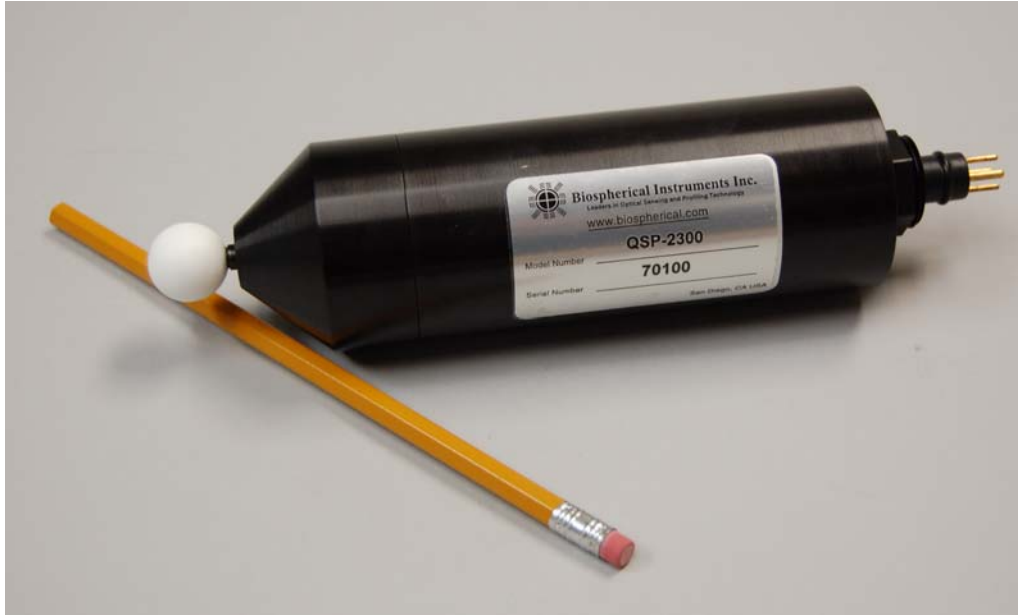
Figure 1. QSP-2300 Quantum Scalar irradiance sensor. The output of this device is a voltage that is proportional to the log of the scalar irradiance.
