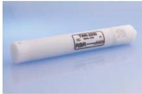
Models TGR-1050P, TGR-2050P and TWR-2050 are autonomous instruments which are intended to be mounted on the sea bed. They will record to internal memory for periods of up to two years, and contain 8Mbytes of flash memory. Temperature is measured in the 2050 models.
