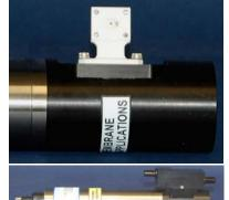
characterization of the internal sensor temperatures that control these processes, especially when water temperature is changing rapidly, is a key accomplishment of the design. Not only does the SBE 43 sensor measure temperature in the right place: the temperature equilibration time of the entire sensor head has been reduced to a few seconds, so it tracks changing water temperature much more faithfully.
