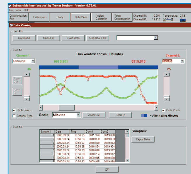
Figure 2. The Data View screen allows the user to download and view data from the internal data logger, as well as view data from real-time data transfer and saved files.
