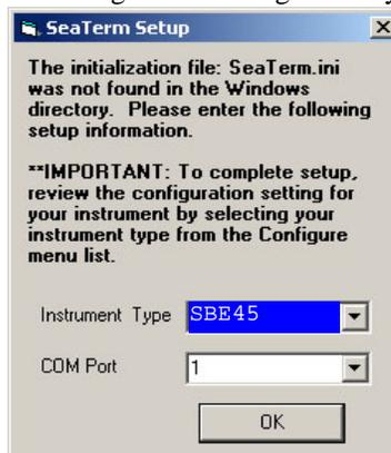
Select the instrument type (SBE 45) and the computer COM port for communication with the MicroTSG. Click OK.
