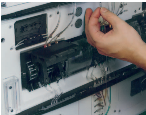
Quick-connect strips make changing the tubes faster and easier
