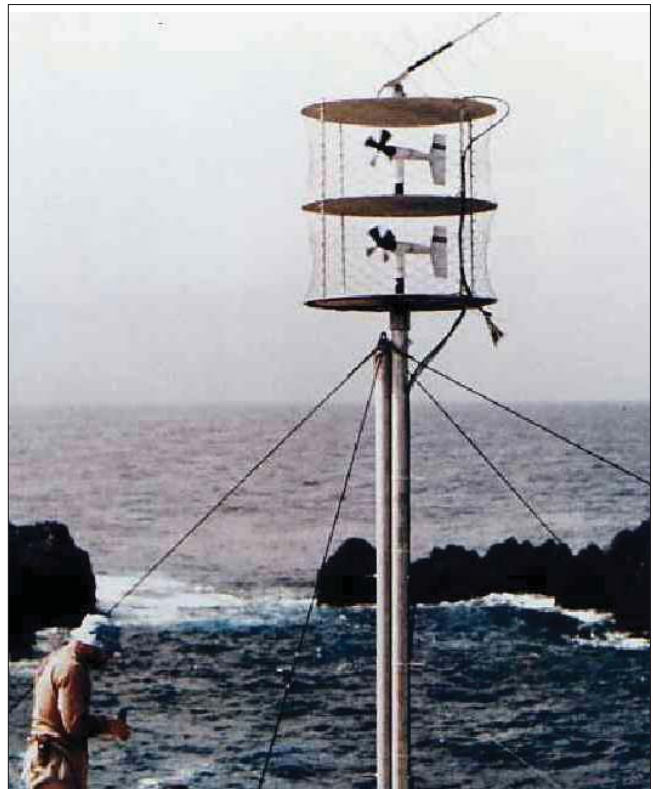
An innovative method of discouraging interference from birds was used at a station at St. Peter and St. Paul Rocks (Brazil). Photo courtesy Dr. Silvia L. Garzoli (Director of the Physical Oceanography Division of the Atlantic Oceanographic and Meteorological Laboratory of NOAA).
