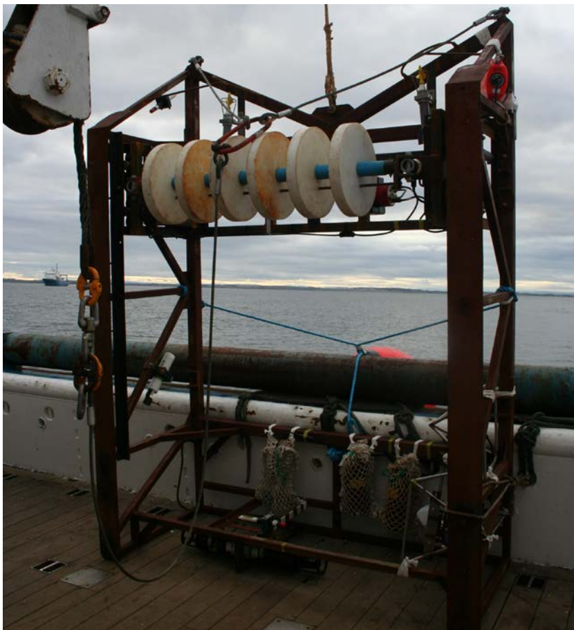
Figure 2: The Bigg sledge with towing bridle and lifting line attached, the ground gear being tested is 400mm discs in the “spaced” arrangement.
