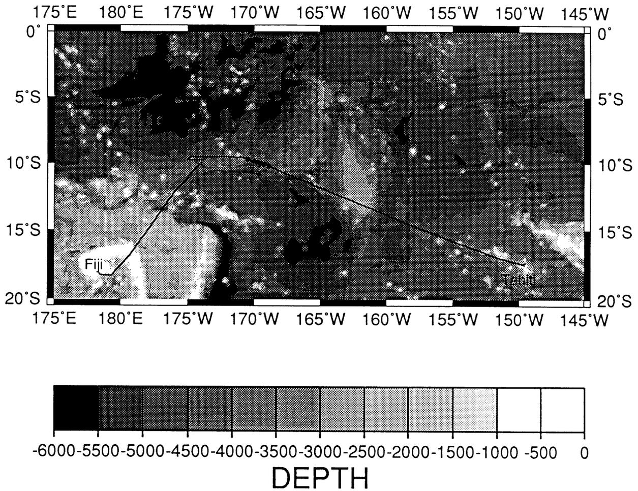
**Figure 1.** Ship track superimposed on ETOPO5 bathymetry. The cruise went from Fiji to Tahiti via the Robbie Ridge and the Samoan Passage. The circles are moorings in the Samoan Passage. The Manihiki Plateau is the shallow feature at about 9°S, 162°W.
