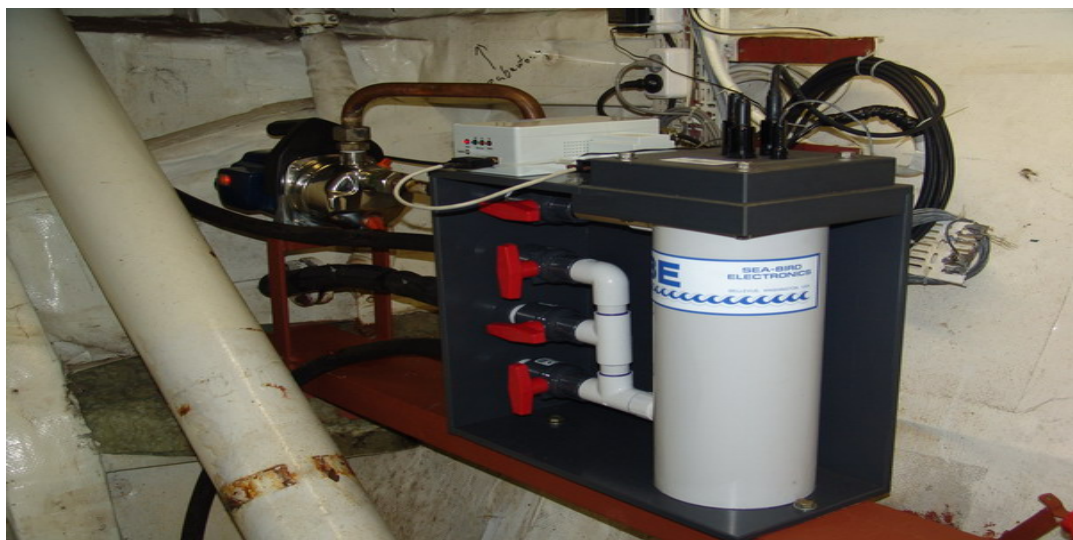
Figure 4. Thermosalinograph SBE 21 aboard of R/V Akademik Ioffe.
