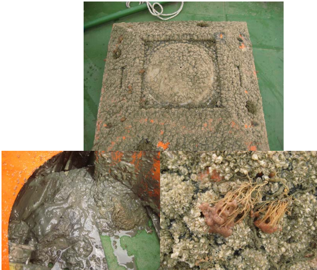
Photo of ADCP recovered at MOW1 and fully covered by biofouling.
