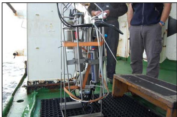
Fig 3. The TriOS-microFlu sensors were mounted in a special frame onto the SeaCat
