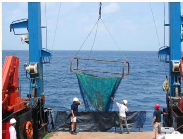
Fig. 1. The Agassiz trawl in action during CD146.
