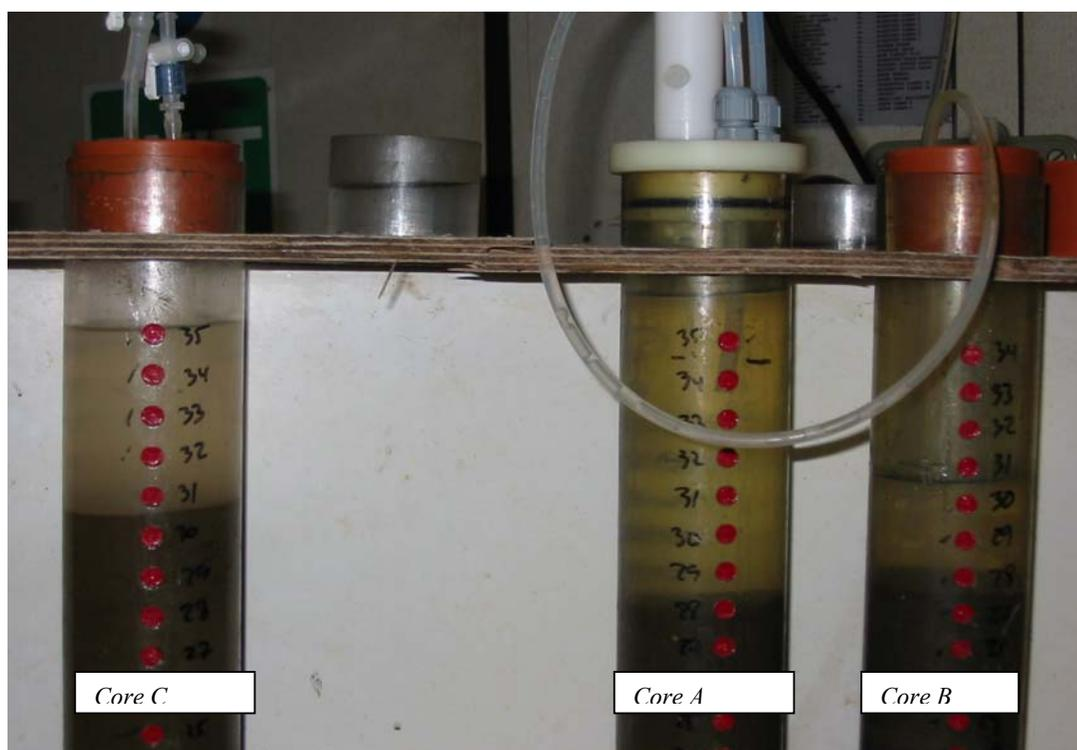
**Figure 2.** Acetylene block cores
