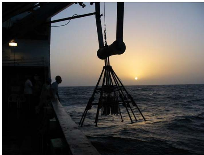
**Fig. 1.** Multicorer deployment from the starboard gantry at sunset.
