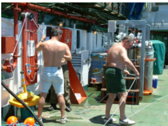
Assembling a drifter buoy with a 180 metre long thermistor chain attached.
