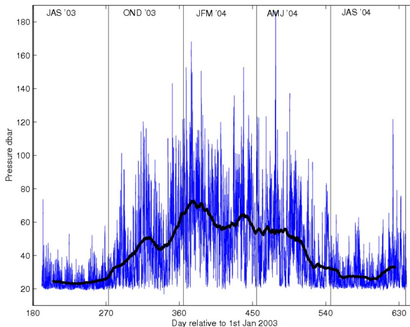
*The pressure record from the upper Microcat of TUBE 12 (blue: 10 min samples, black: 28 day running mean)*
