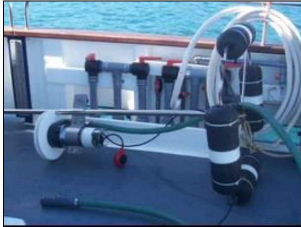
Figure 3.1.4 Near-surface zooplankton pump
