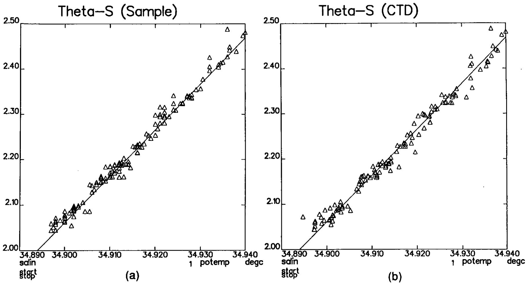
Figure 3 Theta-S plots for Cruise 189 sample data (a), and CTD data (b). CTD data are CTD salinities corresponding to closure of Niskin bottles. The straight lines show the Saunders (1986) relation.
