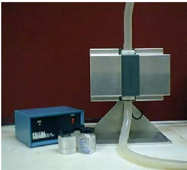
**Fig 6.18.1 Laboratory OPC and Deck Unit for use in pump-through mode for continuous underway or discrete net samples.**
