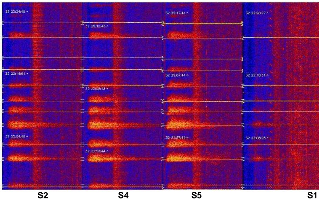
Screenshot of the spectrograms of the signals recorded by four Sirena hydrophones (time increases from bottom to top). The signals originate from an earthquake swarm on the Reykjanes Ridge
