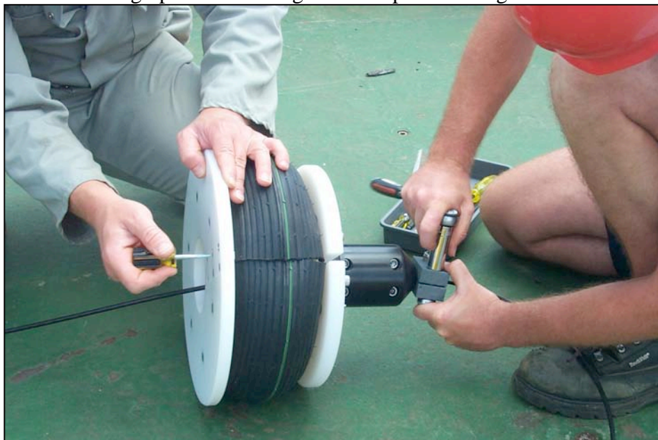
Photograph 4: Attaching MMP stop to mooring wire
