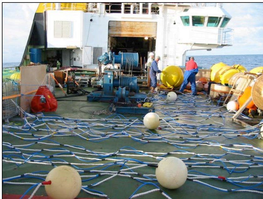
Photograph 7: EB3 inductive mooring umbilical flaked on deck prior to deployment
