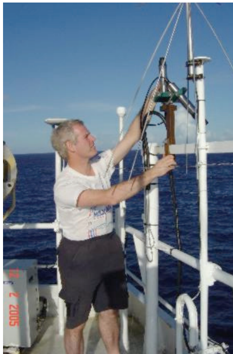
Figure 29 : Hyperspectral radiometers were attached to the starboard side of Monkey Island on RRS Discovery, giving the downward-looking one a clear view of the water ahead of the ship's wake.
