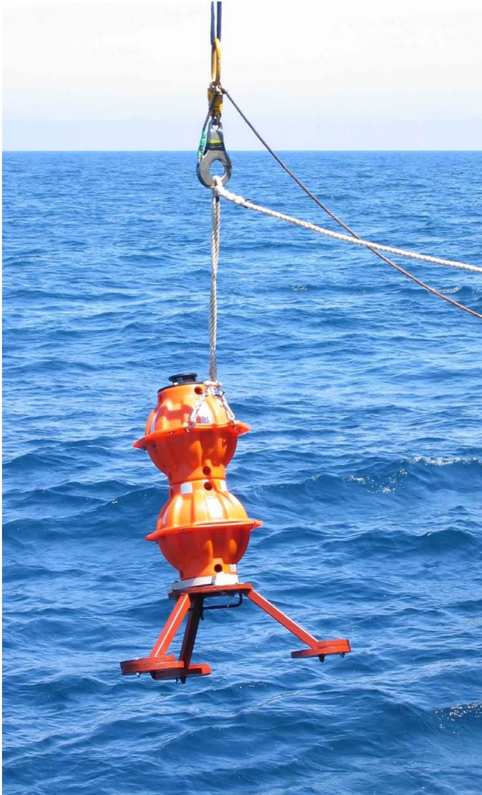
Figure 6: Deployment of a Lander BPR.
