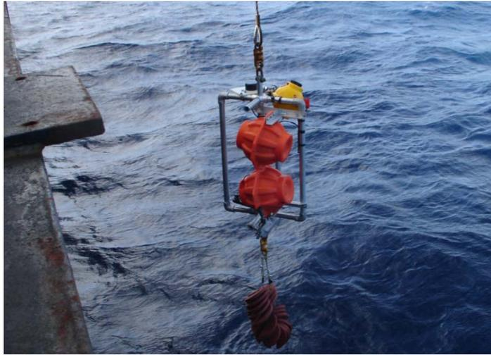
c – Frame Deployment for Glass Spheres, Benthos Acoustic Link and Modified Release Assembly
