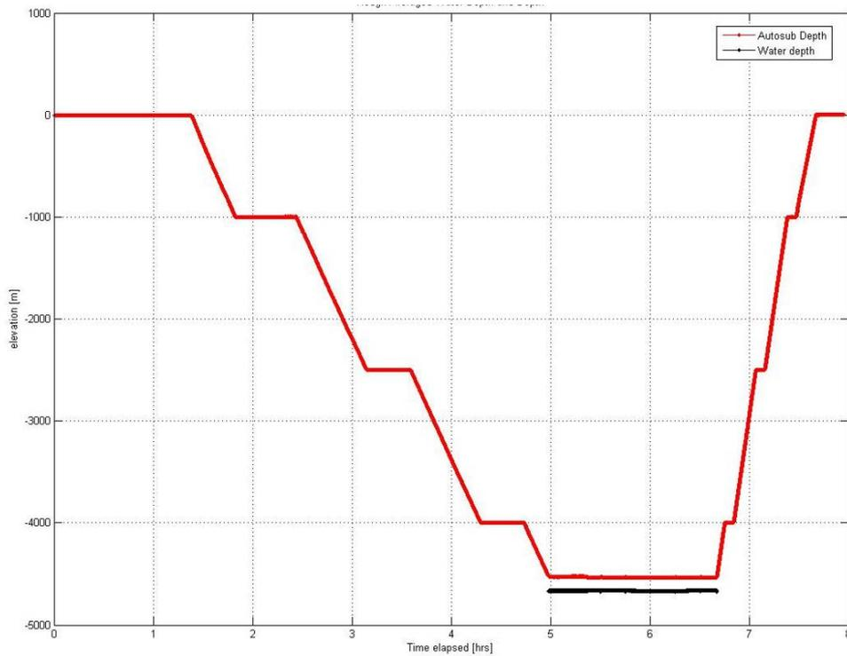
Figure 3. Depth profile for the Autosub6000 first deep water mission (the 2<sup>nd</sup> ever deployment of the AUV) The red trace is the AUV depth, the black trace is the seabed depth as measured by the AUV's ADCP.
