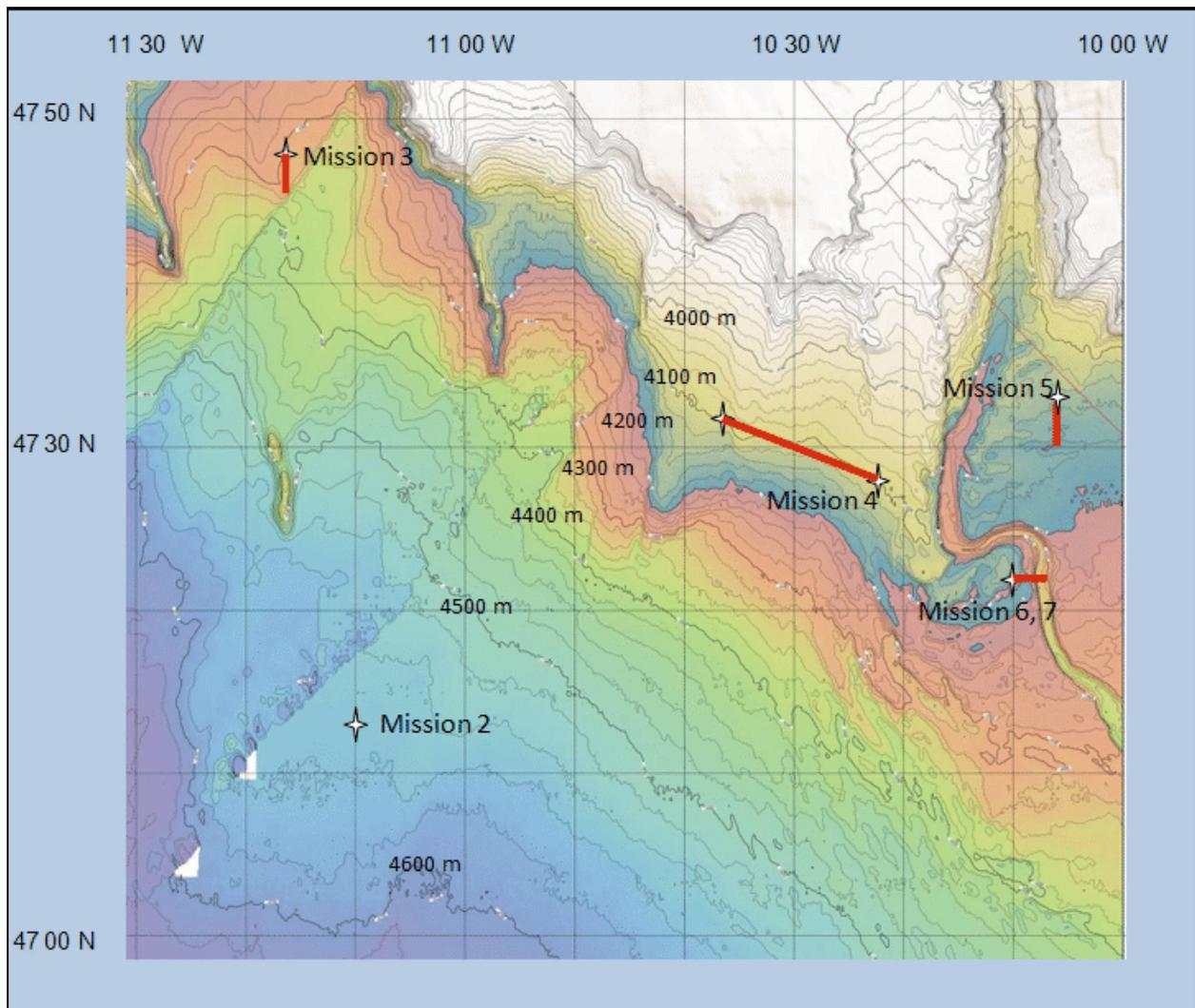
*Figure 1. Map of the Operating Area. Autosub Mission 1 was in Falmouth bay, Mission 8 was in shallow water to the north east of this chart, for navigation test runs. Bathymetry provided by UNCLOS group, NOC. data sources are UK Navy, Irish National Seabed Survey (Geological Survey of Ireland) and Petroleum Affairs Division, Ireland.*
