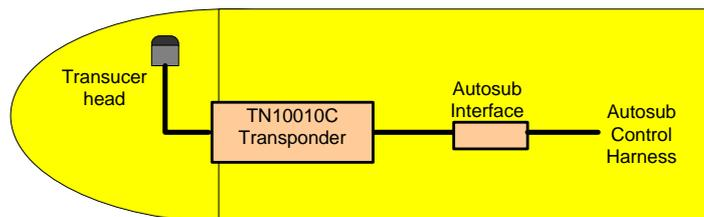
*Figure 6. Ship side and AUV side block diagram.*
