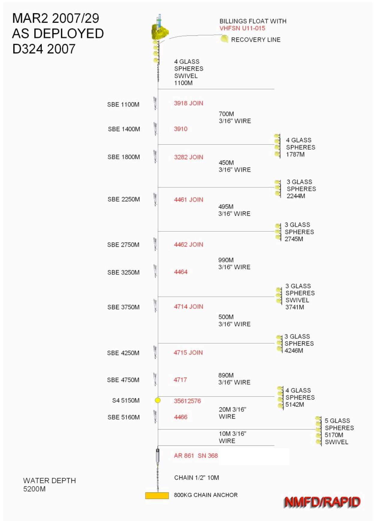
Figure A.17: Mooring diagram of MAR2 as deployed on D324
