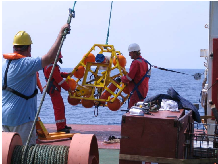
Figure 10.2: NMF low-profile ADCP lander being recovered at IM2
