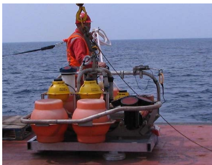
Figure 10.1: 150kHz ADCP lander ready for deployment at WIS.
