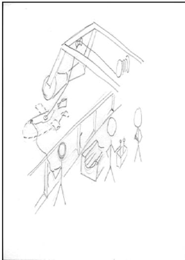
*Fig 6. Schematic of the recovery once the ALR recovery lines have been attached to the winch line. Note the winch line passed over the FAR side of the roll to keep the ALR at some distance from the ship, not the near side as drawn.*
