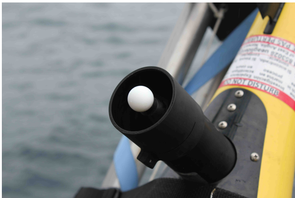
Figure 32: Photograph of the PAR shield attached before deployment.
