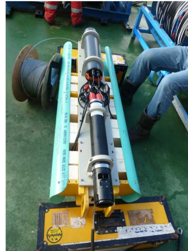
Figure 13: Wirewalker setup without side guards and floats (left). Wirewalker setup on mooring wire and ready for deployment (right).
