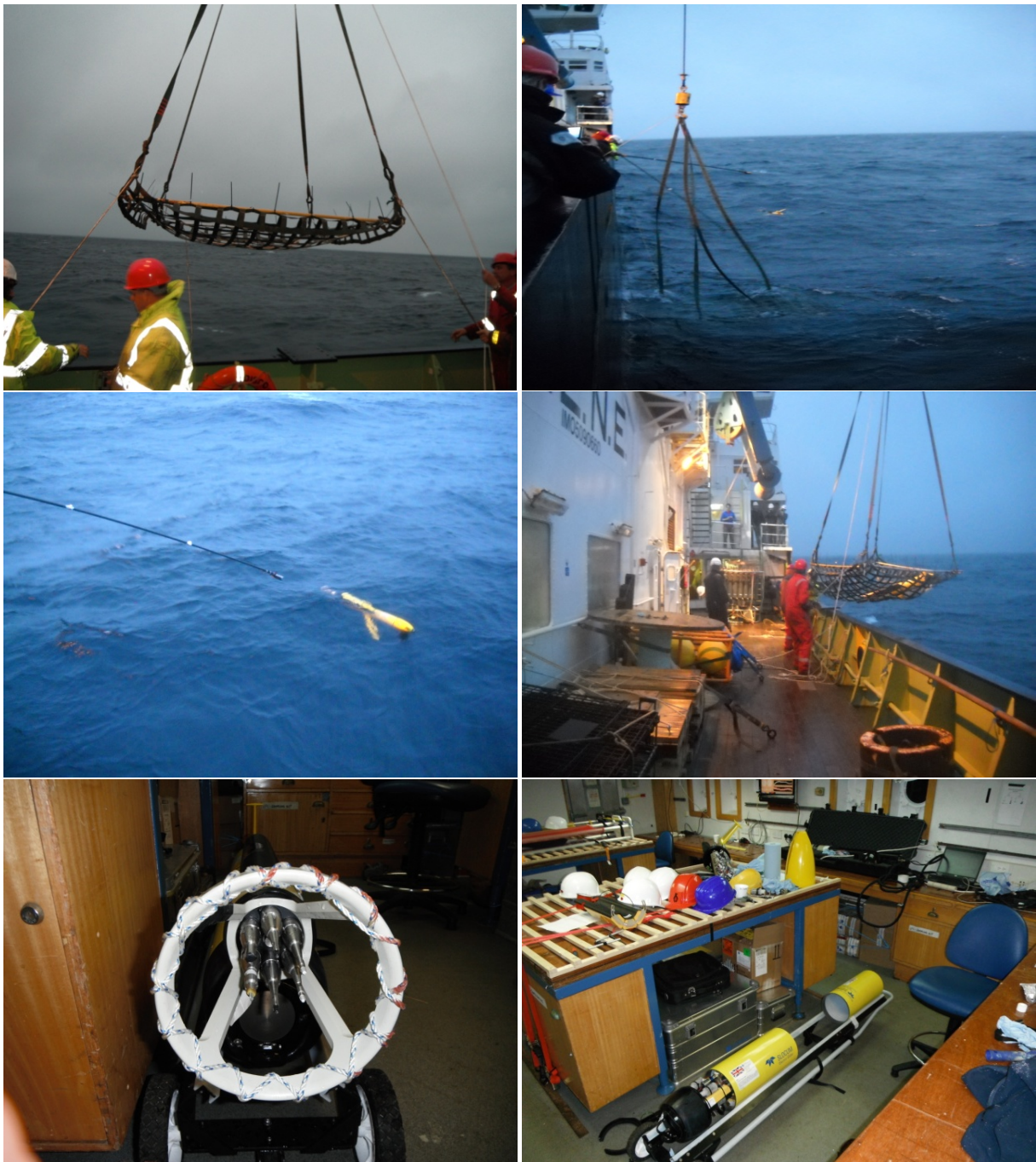
Figure 19: Turbulence glider recovery operations. Recovery net deployment (top right). Glider alignment for recovery (top left). Port wing lost after first recovery attempt (middle right). Glider recovery. The sea swell and white cap can be seen in this picture just below the recovery net (middle left). Turbulence probes clean and intact after the recovery (bottom right). Servicing of the recovered glider (bottom left).
