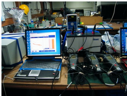
Figure 2. YSI ProODO optodes deployment and the water bath used.
