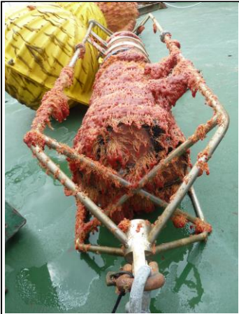
Bio-fouling on ADCP S/N 3725 was particularly bad
